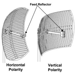
grid as shown for optimal antenna performance.
