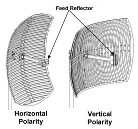
Important Note: Feed Reflector must be orientated to grid as shown for optimal antenna performance.
