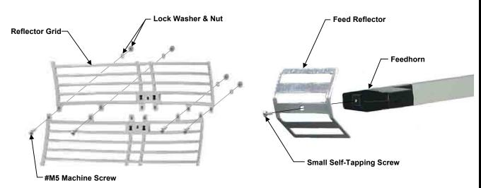
Assemble the halves of the Reflector Grid using (4) #M5 machine screws with lock washers, flat washers and nuts as shown.
